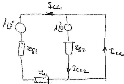
$$\bar{I}_{cc1} = \frac{1 \angle 0^\circ}{Z_{12} + Z_{11}} = \frac{1 \angle 0^\circ}{0,15j + (0,15 + 0,1125j)} = \frac{1 \angle 0^\circ}{(0,15 + 0,2625j)}$$
