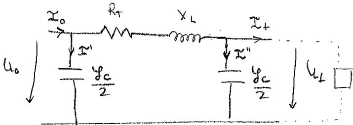
$$U_t = \frac{220 \cdot 10^3}{\sqrt{3}} \angle 0^\circ \quad \text{Asignamos ángulo } 0^\circ$$
