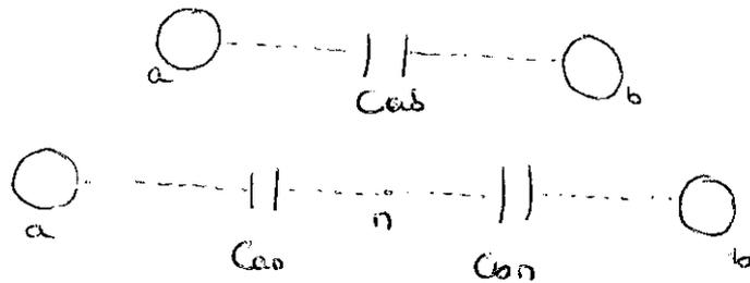
$$C_{an} = C_{nb} = \frac{2\pi\epsilon}{\ln \frac{D}{r}} \text{ (F/m)} \quad (C_{an} = C_{nb} = 2C_{ab})$$
