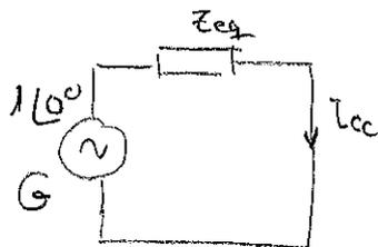
$$Z_{eq} = \frac{\bar{Z}_1 \cdot \bar{Z}_2}{(\bar{Z}_1 + \bar{Z}_2)} =$$
